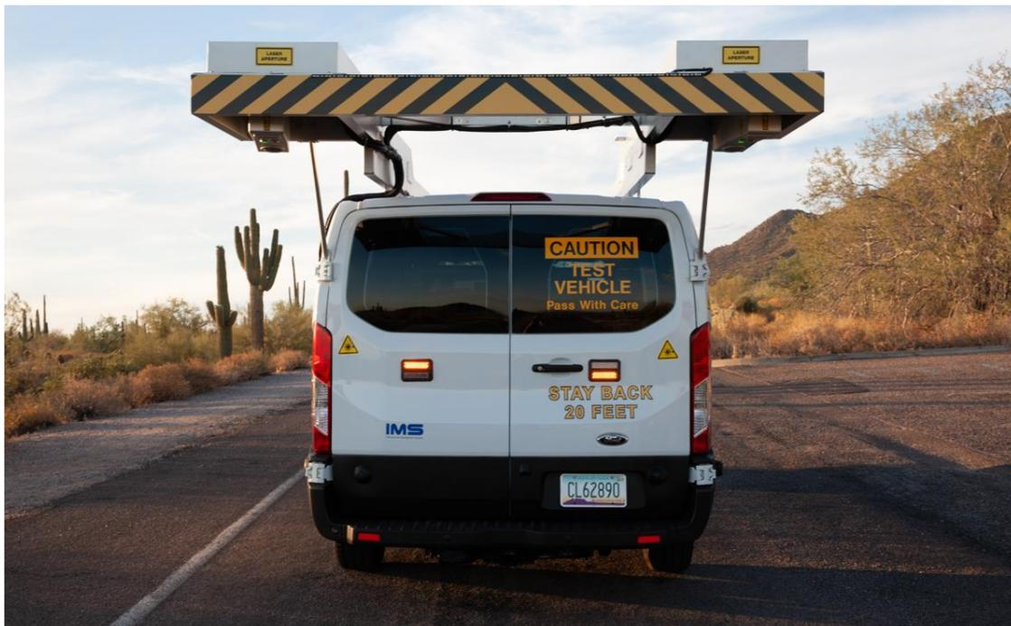
**Figure 9 - LCMS2 data collection vehicle**
