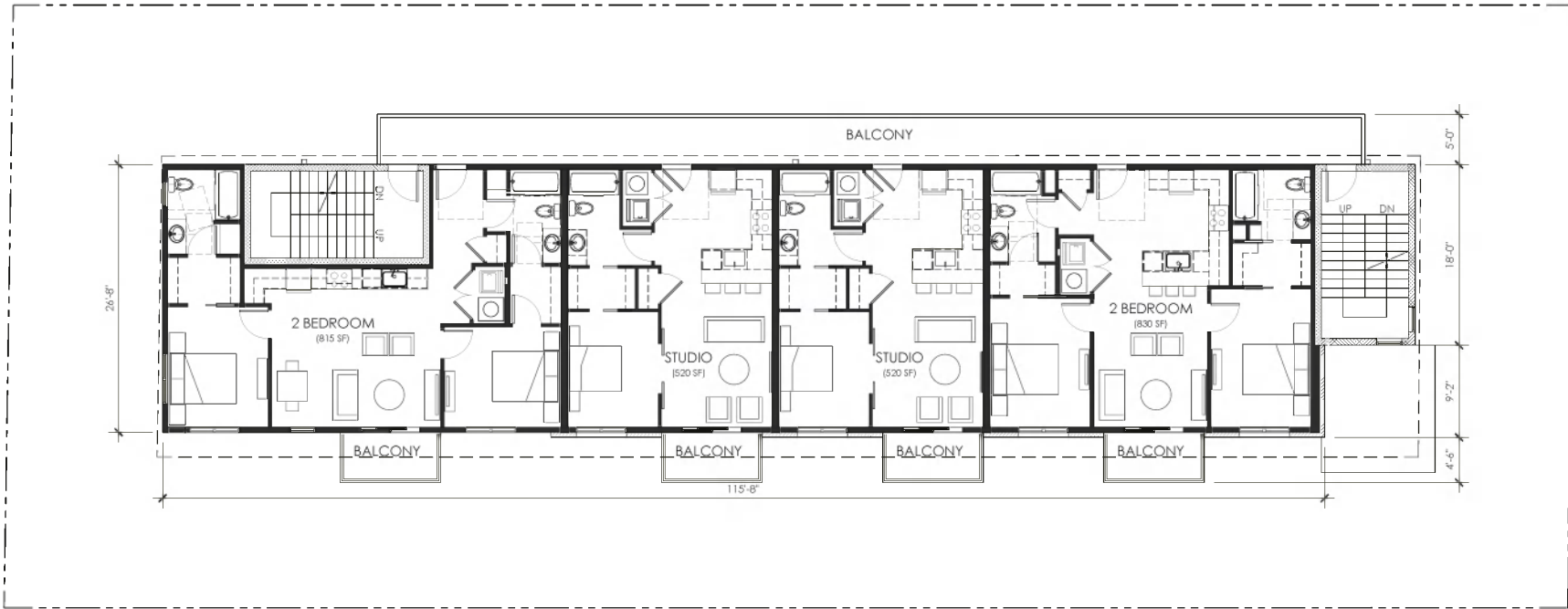
01 SECOND FLOOR PLAN A2.2 SCALE: 3/16" = 1'-0"
